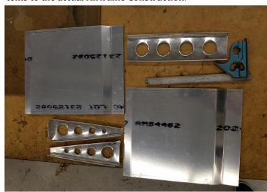
The evening Airframe class has been working on a cool project. The project was designed by NVOC Aviation Instructor, Mr. Perkins. The project involves fabricating an airfoil shaped section of a wing from a blue print. To accomplish this, a student will take a flat piece of 2024 T3 Alclad Aluminum, cut, bend, drill, and shape it into several flat pieces.
