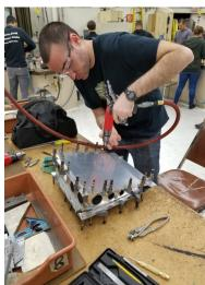
The main part of this assembly is what is called the rib of the wing. These ribs are flat pieces that have holes drilled in them to save weight. These ribs are then assembled together and riveted into a structural component many times stronger than the original piece of sheet metal. See a counselor for more information about the Aviation program.
